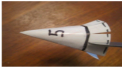
3. Cut nose cone edge into 5-8 flaps
