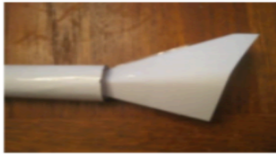
1. Slide nose cone into body tube
