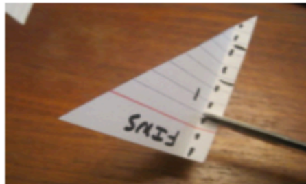
3. Mark and cut 4 equal flaps into fin
