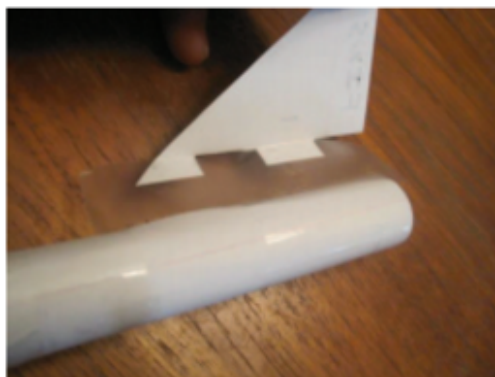
2. Align fin parallel to body tube and tape/glue in place
