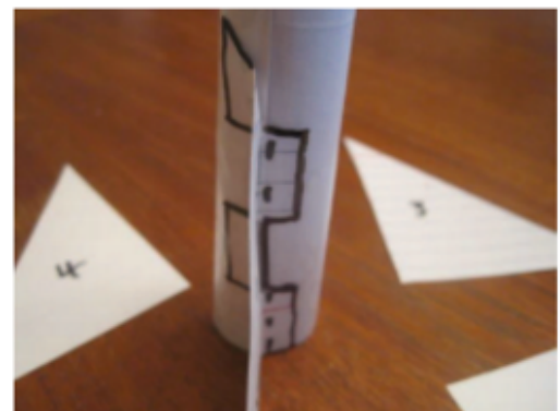
3. Check fin parallel is aligned straight in vertical directions. Tape/glue the additional fins equally around body tube
